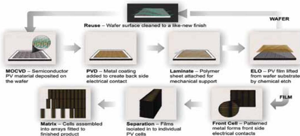
Figure 2 | Solar cell manufacturing process
