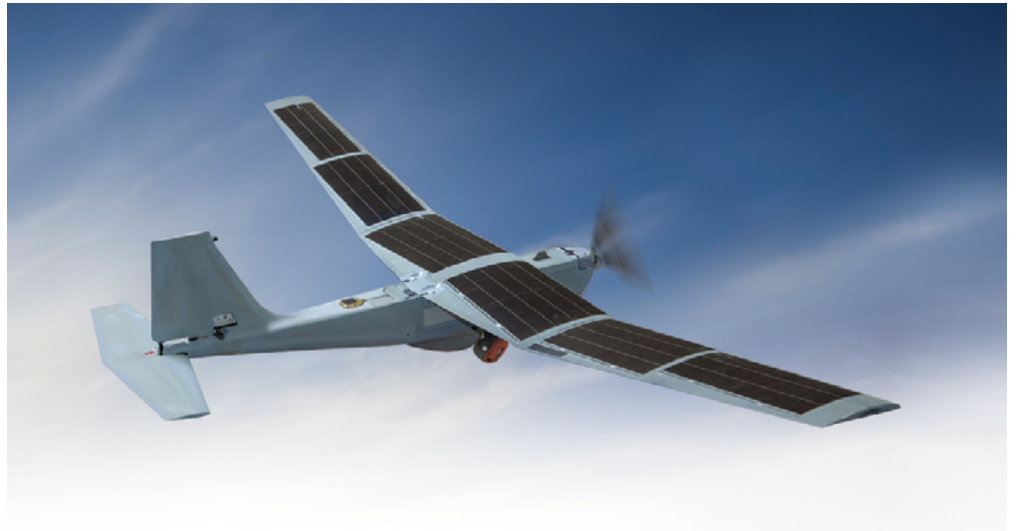
Fig. 1. Solar cells can help quadruple the range of battery powered UAVs.
