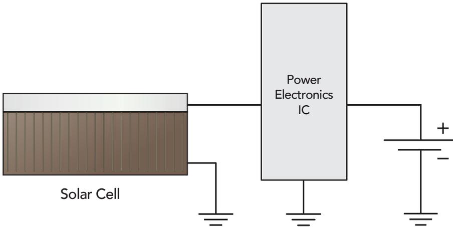
*Fig. 4. Battery Replacement Block Diagram*
