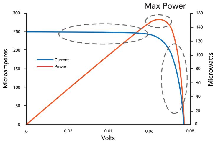
*Fig. 3. Low Light IV curve and Maximum Power Point*
