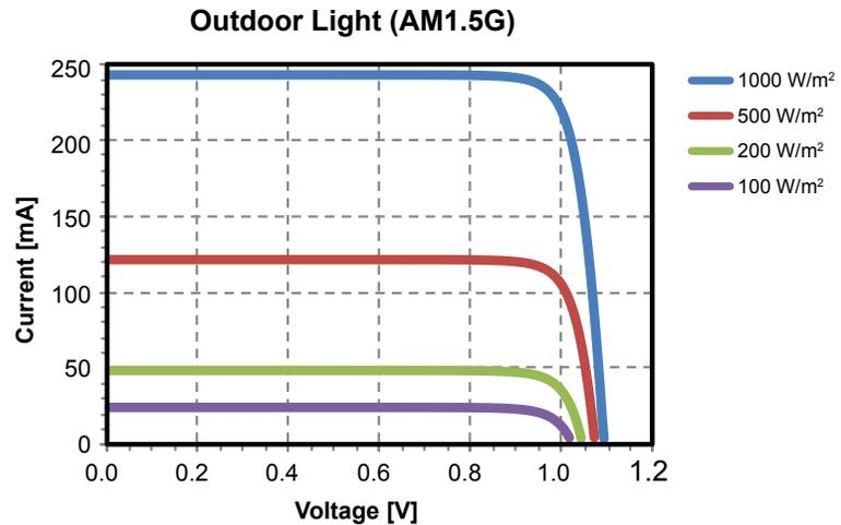
Fig. 2. The Current versus Voltage (IV) curve
