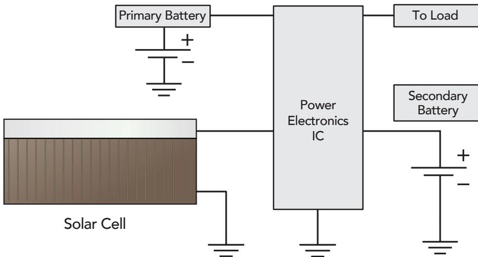
*Fig. 5. Battery Extension Block Diagram*
