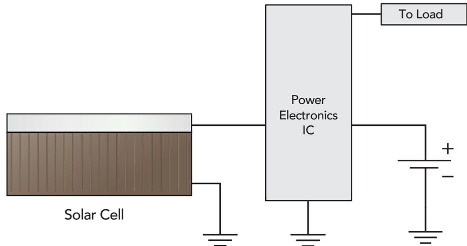
*Fig. 6. Integrated Regulated Output Block Diagram*
