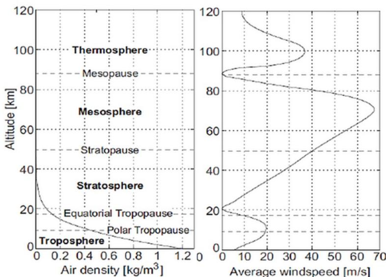
Figure 1. Air density and average wind speeds vs. altitude. The preferred altitude for high-altitude pseudosatellites is 20-30 km, in the zone of low wind speeds. Air density at 20km is roughly 1/10 that at sea level.<sup>3</sup>
