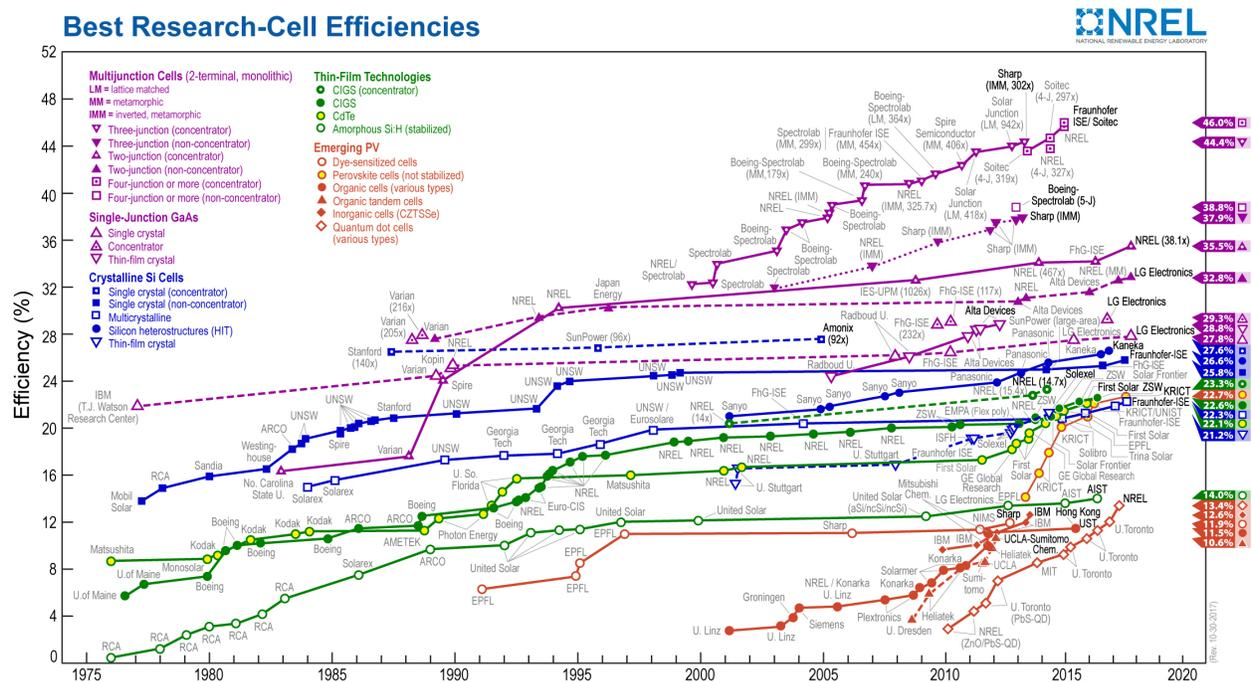
Figure 3. Evolution of solar cell technologies and efficiency records. There are now over 20 cell technologies being actively developed by researchers globally, and being tracked by the National Renewable Energy Laboratory.<sup>5</sup>
