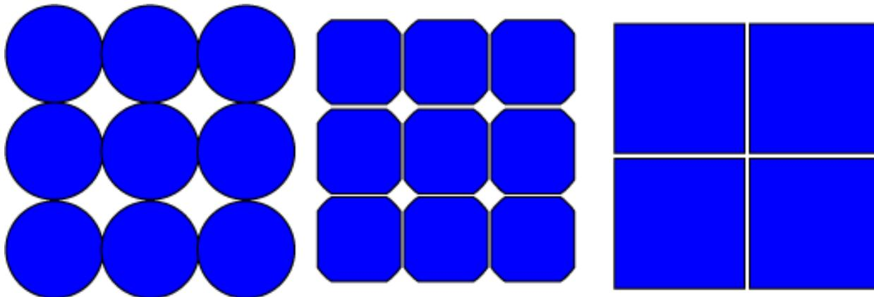
Figure 2. Solar cell packing factor, the ratio of actual solar cell area to the available area, depends on cell and interconnect design. Wing shape can also be a factor.<sup>4</sup>
